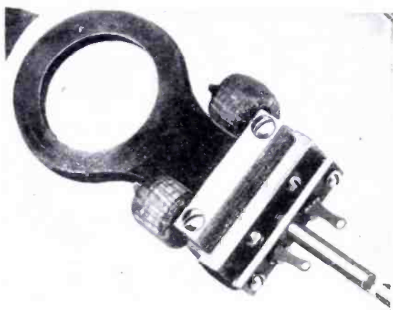
Fig. 6—At left, shows adjustable magnet mounting, forming a part of the special synchronizing motor as shown also in Fig. 5. A toothed rotor rotates between the poles of the two magnet coils and acts to preserve synchronism.
