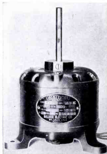
Fig. 7—Shows appearance of the special vertical type, scanning drum motor.
