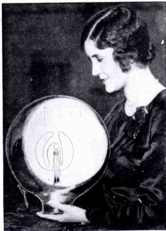
Here we see the relative size of one of the huge photo-electric cells used at Chicago transmitting station W9XAO.
