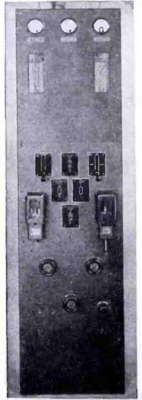
Fig. 6—Power supply unit for Columbia television transmitter.
